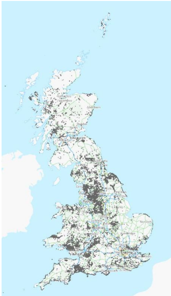
Fig 1. Spatial distribution of GB landslides – BGS National Landslide
