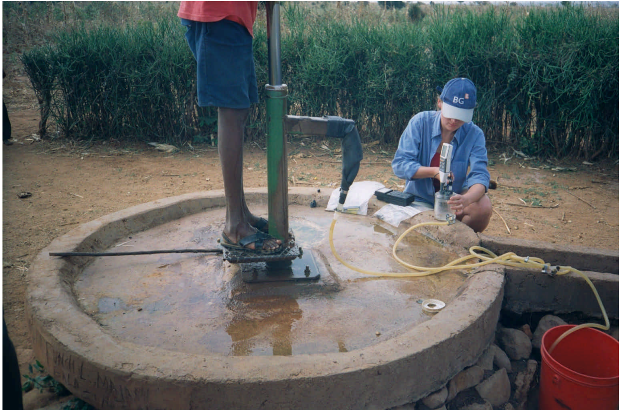
Figure 4 Sampling procedure for making an airtight connection for taking flow through cell measurements and CFC samples from a Nira handpump.
